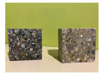
Concrete with (left) and without pyrochar: One part pyrochar reduces three parts CO<sub>2</sub> of the overall product.
