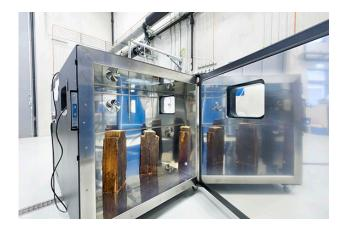
The CycloPlasma process for decontaminating building materials containing PCP and lindane.
