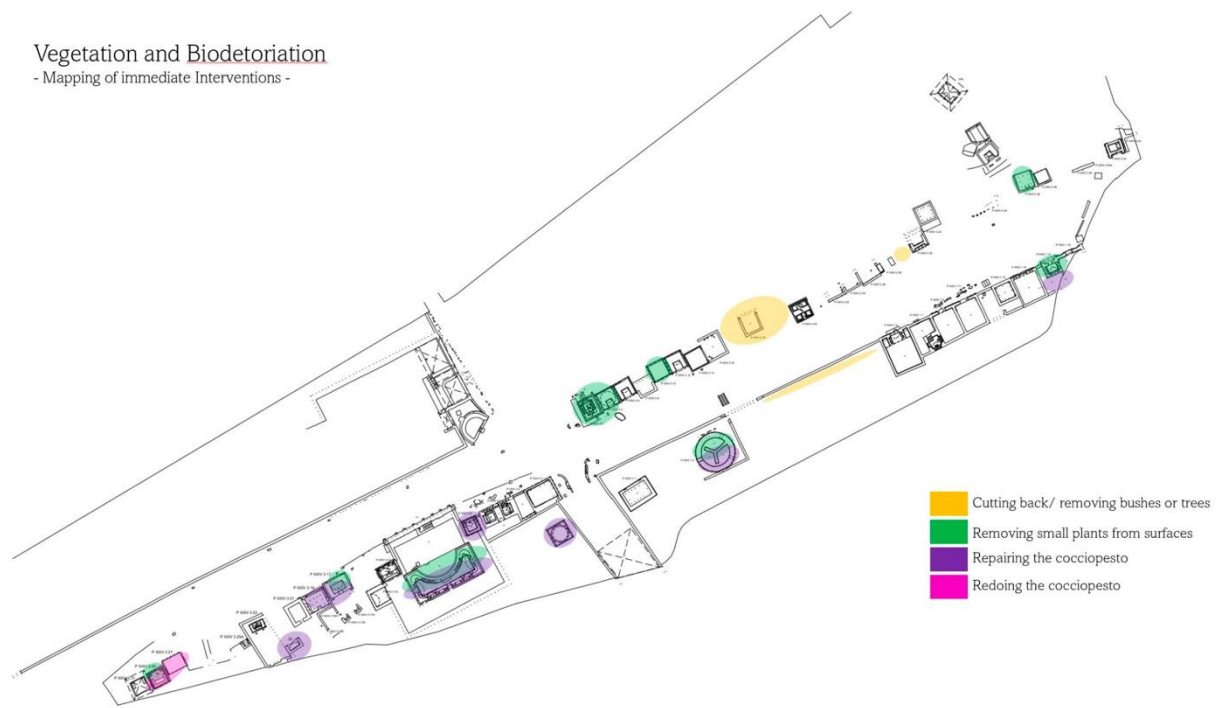
Figure 8 Map of immediate interventions concerning vegetation and biodeterioration developed by the participants
