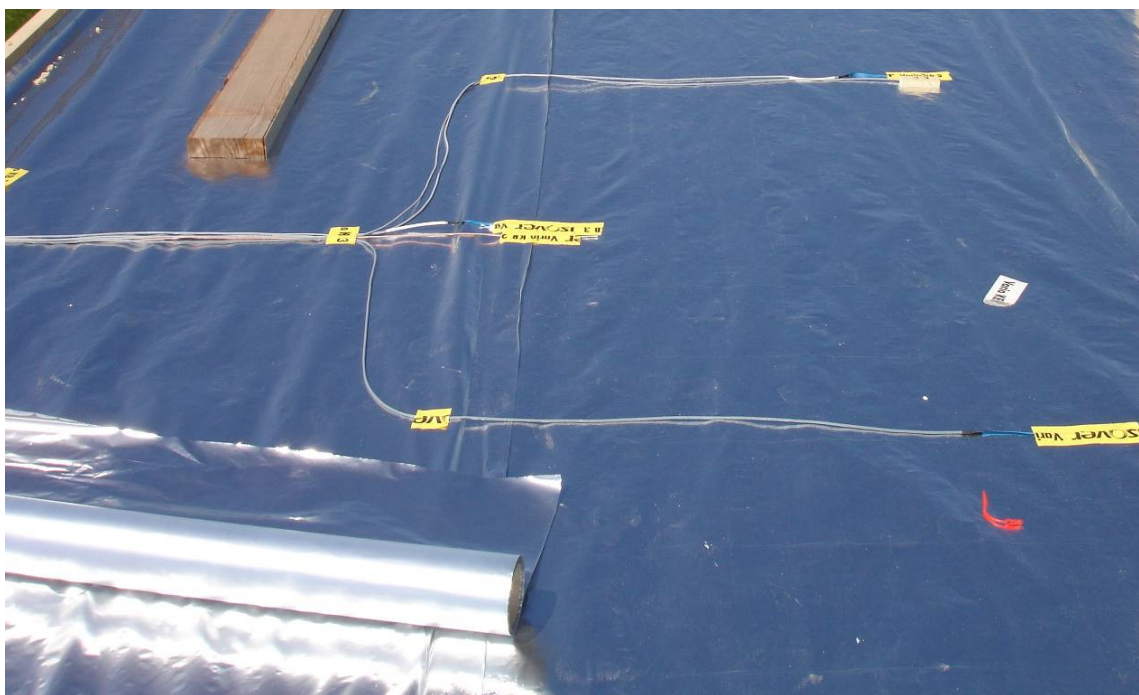
Figure 6: Installation of the interior sensors (below the glass fibre boards) for RH and temperature measurement. In the middle, a PT100 is combined with a capacitive RH sensor. Additional PT100 sensors, one combined with a wood moisture sensor, can be seen at the top and bottom of the photograph.
